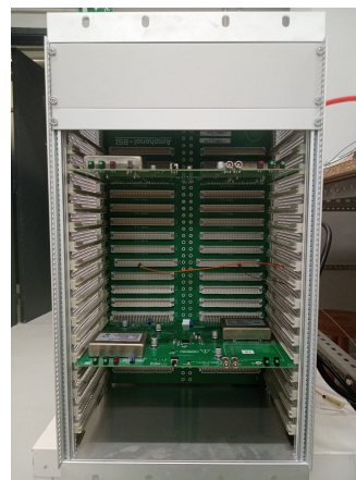
Figure 1. Crate with two connected HVSupply boards on slot 2 and 13.
