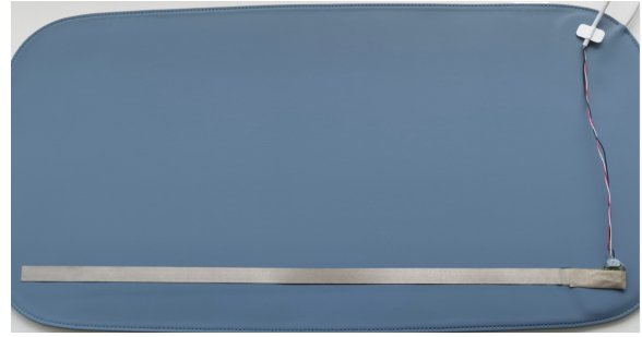
Fig. 5. The monitoring pad and the unencapsulated piezoelectric sensors. The sensors are already placed in their related encapsulation positions.
