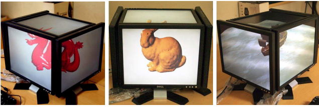
Fig. 15. LCD based display showing various static and dynamic scenes
