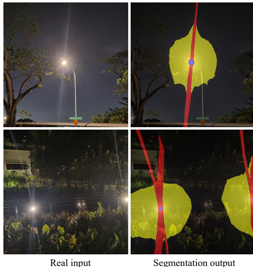
Fig. 17: Lens flare segmentation with our dataset. Since our dataset provides separated images for each component, it can be used for lens flare segmentation. This figure shows that PSPNet [45] trained on our dataset with annotations can accurately segment different components in real-world flare-corrupted images. In this figure, red, yellow, and blue represent streak, glare, and light source, respectively.
