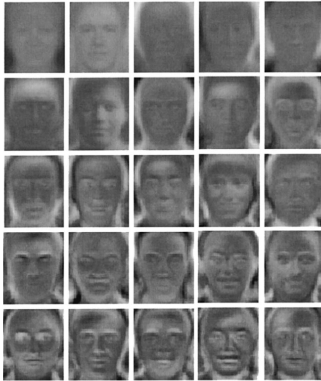
Fig. 9. First 25 PC axes of the image set (columns of P ), ordered left to right, top to bottom, by the magnitude of the corresponding eigenvalue.
