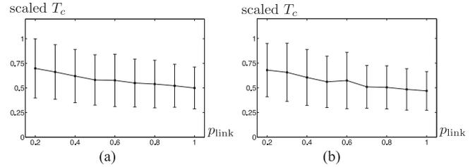
Fig. 8. Error bar plots for the mean convergence time of 100 random realizations, as a function of the link probability of the Erdős–Rényi observation network. The errors are set to be the standard deviation of the convergence time. Fig. 8(a) depicts the realizations for the assign/appraise dynamics, while Fig. 8(b) depicts the realizations for the assign/appraise/influence dynamics. (a) Assign/appraise. (b) Assign/appraise/influence.
