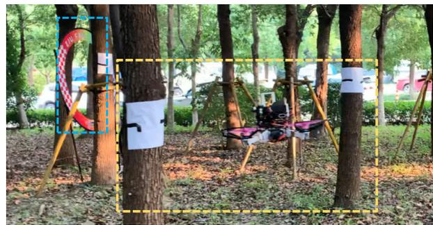
Fig. 15: Flight in forest, the blue box marks a ring and yellow box marks a gate made from two trees pasted with white paper.
