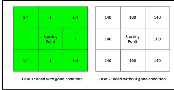
Figure 3. Different assignment of g(n) cost value to different pixel points (Case 1 and Case 2).
