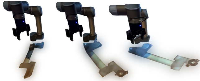
Fig. 3: Dynamic signal: A virtual robot (bottom) moves ahead of the real robot resulting in a brief window for visualization of future motions.
