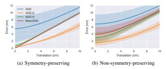
Fig. 8: Error metrics ( $\pm 1$  standard deviation) between object poses with random rotations and increasing translation. ADD-H closely approximates MeanSSD.
