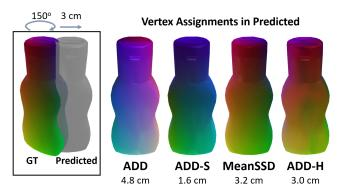
Fig. 7: Pairwise vertex assignments (shown by vertex color) between ground truth (GT) and predicted model poses using four different metrics.
