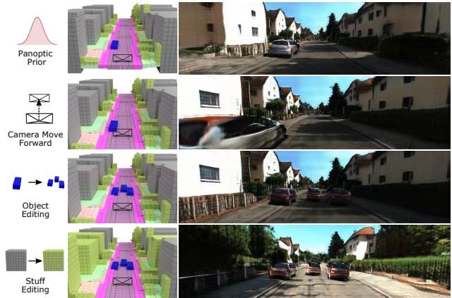
Figure 1: Illustration. UrbanGIRAFFE generates a photorealistic image given a sampled panoptic prior in the form of a semantic voxel grid and object layout. Our method enables diverse controllability regarding camera pose, instance, and stuff.
