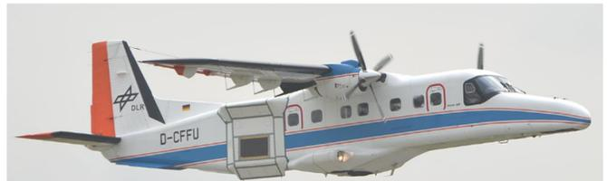
Fig. 2: DLR's aircraft with the SAR equipment (rectangle at the back of the plane).
