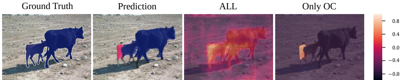
Figure 8. Loss spatial map visualization of OCR with different pixel selection strategy. "ALL" denotes we select all of the pixels to attend the calculation of OCR loss. "Only OC" means only the OC pixels are selected to attend the calculation of OCR loss. "ALL" pixel selection strategy provides unnecessary supervision signals to IC pixels, which causes suboptimal performance. "Only OC" strategy is highly selective to OC pixels, which can efficiently suppress OC error phenomenon for better performance. Blue denotes " cow " and Pink denotes " horse ".
