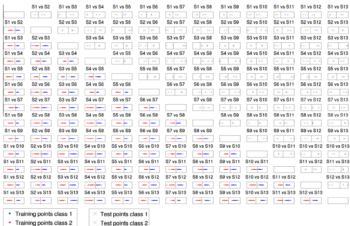
Fig. 9. Decision boundaries (black lines) obtained by the PCA + LDA model for all the pairwise classifiers corresponding to classify one subject vs other ( S_x vs S_y ) in one of the training/test partitions of our evaluation method. Training and test points of the partition are also shown. Best viewed in color.
