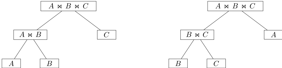
Figure 1.1: Two different join orders for three relations. The left plan joins relations A and B first, while the right plan joins relations B and C first. The order of the joins can affect the cost estimates produced by a cost model.
