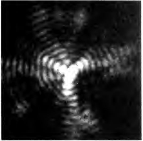
Fig. 3: Laboratory point spread function (simulated spherical aberration and HST FOC f/288 pupil function)
