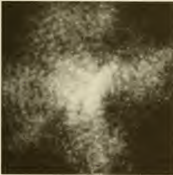
Fig. 4: Laboratory image of the object degraded by spherical aberration and photon noise ( \sim 10000 photon events/frame or \sim 70 photon events in the brightest pixel)
