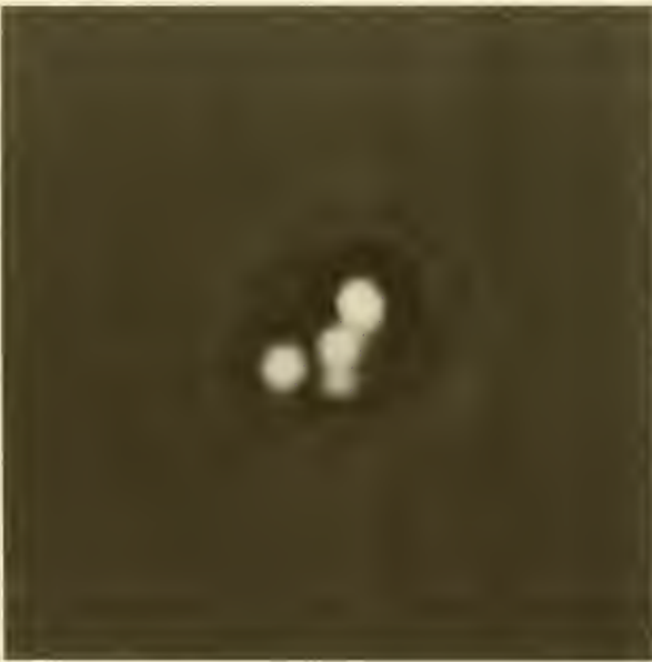
Fig. 8: Image reconstructed from Fig. 4 by the Lucy-Richardson method (140 iterations)
