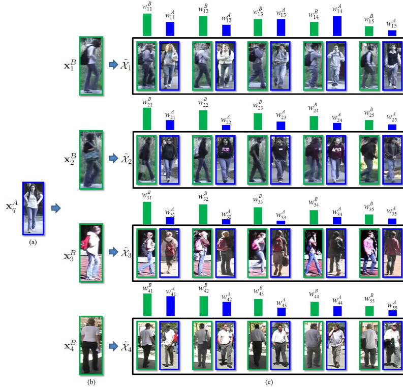
Fig. 2. (a) A query sample observed in camera view A. (b) Samples of four candidate persons observed in camera B based on temporal reasoning. (c) The nearest neighbors of each candidate in (b) found from a large training set by directly matching the visual features observed in camera B. Each person in the training set has a pair of samples observed in both cameras A and B according to manually labeled ground truth. Therefore the paired samples of the found nearest neighbors can be used to train the candidate-set-specific metric. Blue windows indicate samples observed in camera A and green windows indicate samples observed in camera B. w_{ij}^A and w_{ij}^B are the weights assigned to training samples according to their visual similarities with the candidates and the query sample respectively. See details in Section 3.2.
