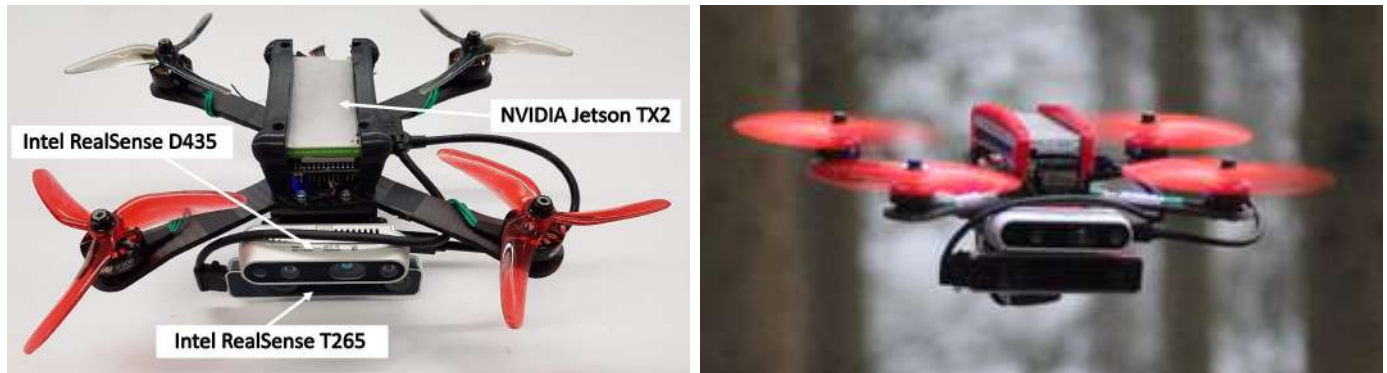
Fig. S3. Illustration of our experimental platform. The main computational unit is an NVIDIA Jetson TX2, whose GPU is used for neural network inference and CPU for the control stack. Sensing is performed by an Intel Realsense T265 for state estimation and an Intel Realsense D435 for depth estimation.
