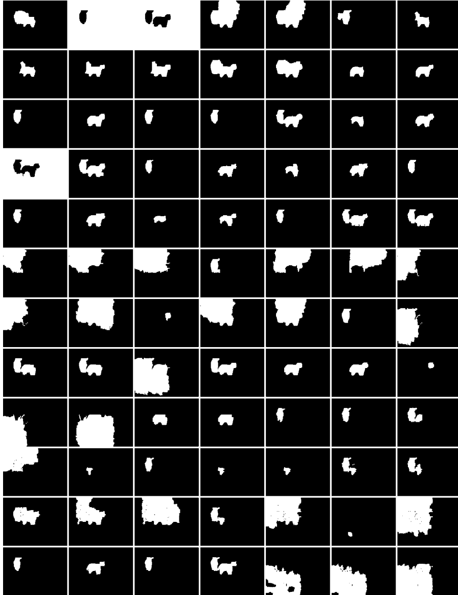
Fig. 4.6 CPMC object proposals for the image in Figure 4.2. Despite the method not knowing what kind of objects are visible in the image, some of the segmentations coincide well with how a human would partition the image into an object and a nonobject regions.
