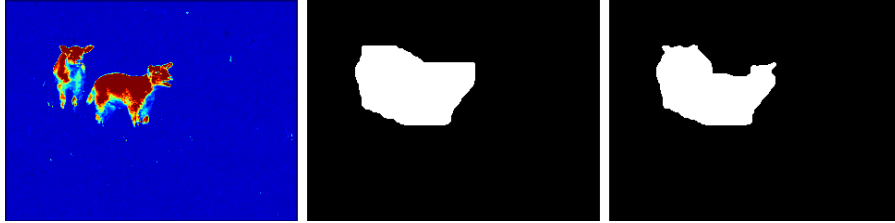
Fig. 4.4 Left: heatmap of unary potential values. Right: segmentation masks for large w .
