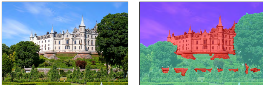
Fig. 6.5 Illustration of Semantic Image Segmentation . Each pixel of an image (left) is assigned a semantic class label, here: sky (blue), building (red), or vegetation (green). Spatial consistency of the labeling is encouraged by pair-wise energy terms between neighboring pixels. (Image source: http://www.flickr.com/photos/foxypar4/3313167875/ ).
